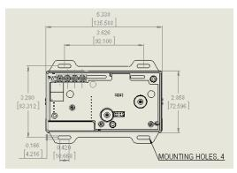
Fig. 3-1 Wall (flush) mount housing dimensions, front view, SRIM1,2
