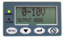
Continue to press the menu key to progress all the way through the menu until you reach the RETURN screen. Press the Enter key to exit out of the menu and return to home screen.
