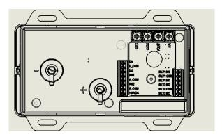
Fig. 3-2 SRIM2 wall (flush) mount housing rear view of pressure fittings and electrical terminations.
